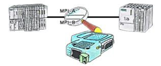
The S7-LAN can also be used for controlling/checking the MPI/Profibus. It will be plugged on the Bus so that you can take a look at the status of the busses via software on PC, for example the numbers of parity errors.
