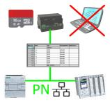
S7-PLC triggered DB-backup/-restore without additional PC via PN-port on SD card
