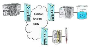
Your pumping stations report the water levels of the central control via telephone network. The central office itself can of course transmit commands/messages to the substations as well. Thereto no dedicated line is required, a "normal" telephone connection is sufficient because the devices cut the line after occured message.
