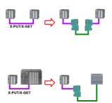
MPI/DP communication between two S7-300/400 controllers on the same bus
