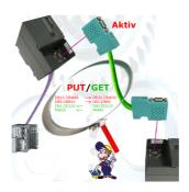
Direct data-exchange between S7-PLCs with S7-LAN.
