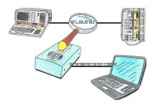
You want check,why your application cant communicate with the PLC or why after some time past the communication will be broken? No problem, integrate the PG-FOX-hardware in this communication way and log through the PG-FOX-software on an PC the sended data in the exact time. So, you can later check the date and find a solution of the problem.
