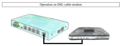
You are looking for a device which can be operated even with DSL? No problem, just plug in your TELE-router to a DSL cable modem, enter the parameters relating to the access data into the device and you are connected to Internet.
