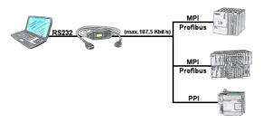
With the MPI/PPI-cable you have the ability to access a connected SPC-PLC S7-200 (PPI 9600 Baud and 19200 Baud) as well as S7-300/400 (MPI/Profbus 9600 Baud up to 187500 Baud) via PC serial with up to 115200 Baud for reading respectively writing of data.
