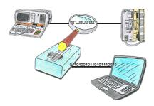
You want check,why your application cant communicate with the PLC or why after some time past the communication will be broken? No problem, integrate the PG-FOX-hardware in this communication way and log through the PG-FOX-software on an PC the sended data in the exact time. So, you can later check the date and find a solution of the problem.
