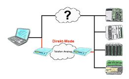
There is an unsupported control or data logger or converter integrated in your installation which protocol is not supported? No problem, the signs that the PC in the office sends will be transferred via telephone line by the Direct-mode , and on-site reproduced by the TP/TB. The way back is identical. So in that case there's also a communication to the electronic devices available.
