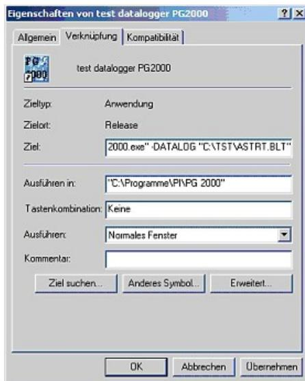
At Destination is the application-name “C:\Programme\PI\PG2000\PG2000.exe“, add following parameter: “C:\Programme\PI\PG2000\PG2000.exe“ -DATALOG “C:\TST\ASTRT.BLT“
