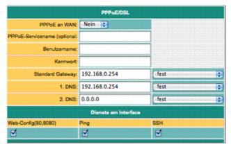
Define here the parameters for operation at a fixed DSL / cable modem. To overview and easier configuration are possible also the default gateway and DNS settings. As a rule, here are to set "auto PPPoE".
