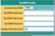
If TeleRouter to be reached by OpenVPN as via the Internet, the Internet IP address of the device must be known. Meaningful here is not to work with a fixed IP address because the provider possibly allocate a new IP address here after new connection establishment (eg via PPPoE). It makes more sense here to access the device always with the same domain name.
