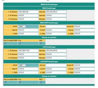
The WAN / LAN port can each receive up to 3 different IP addresses and subnets.
