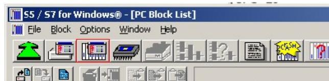
7. Back in the main window press the „PC Block List“ button for testing the new established communication configuration.
