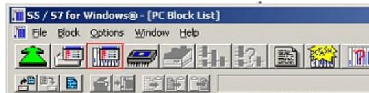
7. Back in the main window press the „PC Block List“ button for testing the new established communication configuration.
