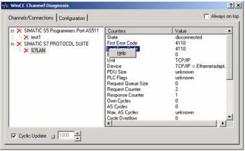
20. The tool could not detect a running connection so it marked the connection/s with a red 'X' (registry card "Channels/Connections").
