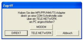
For access query choose "Direct" if your product connects via USB-cable or Nullmodem-cable. "Modem" if your product connects via telephone line or "TELE-Network" if your product connects with a TELE-Network device via telephone line.
