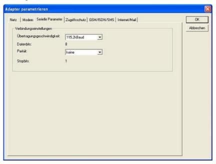
In this dialog the transfer-rate between modem and TS-Adapter is selected.
