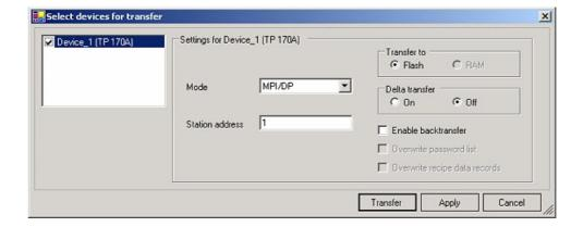
9. Press the button "Transfer" to start communication with the terminal. Your project is about to be transferred.
