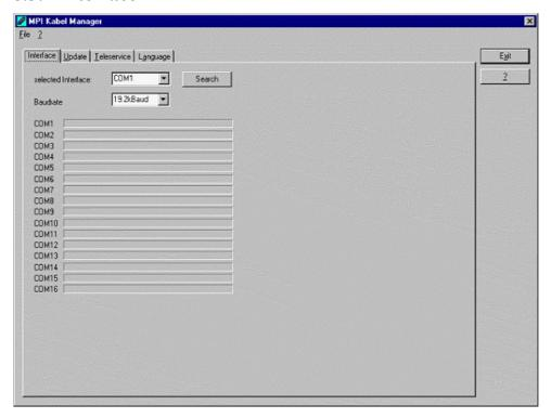
In "set interface" you can choose the COM-port you device is connected at. Only the COM-port which was aktive at starting the MPI-Kabel-Manager are shown.
