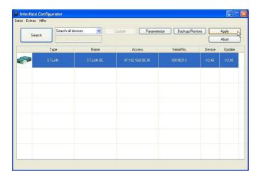
15. Activate the "Automatic-mode" when you will be shure, that the connected PLC sends cyclic busparameter-protocols. When not please configure the bus by hand.
