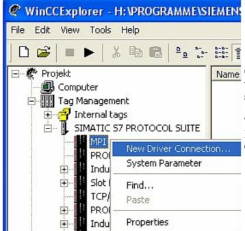
Name 6. For a proper working communication with the PLC there must be defined how the software has to communicate with the PLC
