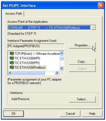
18. If you want to use ProTool/Pro RunTime you can set the "PG/PC Interface" by selecting the entry "DPSONLINE". Therefore you have to select "Access Point of Application" and configure it as described above. The easiest way is to use the S7-LAN/MPI-LAN/MPI-USB- driver which supports USB and LAN products.
