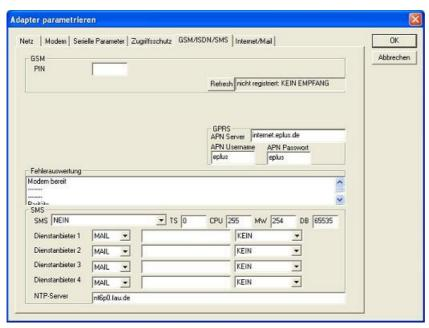
**PIN:** PIN-Number of the SIM-Card, up to 8 numeric chars, (only for TELE-SERVICE GSM).
