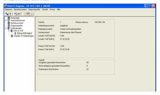
6. Now open the DB100 in your S5 - PLC and the DB10 in your S7 - PLC and check if the values are consistent with those from DW100 of the 20 bytes that you configured in the other PLC in DB100 and DB10 from DW0. If that is the case, the communication between S5 and S7 was successfully completed.
