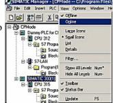
36. To test the communication open the branch of your real existing PLC (e.g. "SIMATIC 300(1)"). The branch below the PLC is the CPU Type (e.g. "CPU 315"). A additional red symbol is displayed next to the standard CPU symbol. Open this branch, too. The next branch you should open is named as "S7 Program" (e.g. "S7 Program(3)"). Finally click on "Blocks" to get a complete list of available blocks from your PLC.
