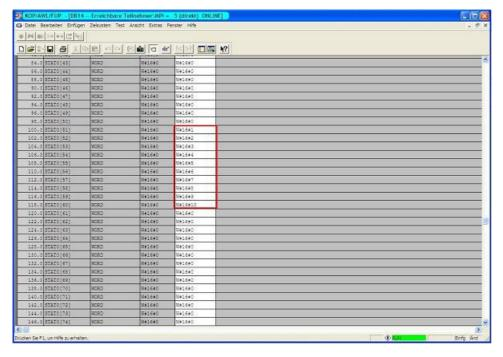
The marked bytes from DW100 should be the same as the ones you have configured in DB100 of the S5 - PLC from DW0.
