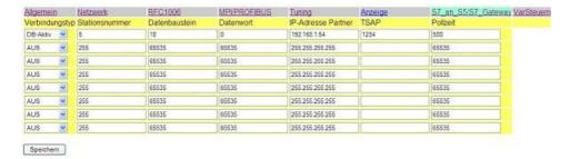
Finally, you still have to see "RFC1006" in "Target - CPU", enter the number of your CPU that is stored is in your PLC and the "Bus" should be set on "Config".
