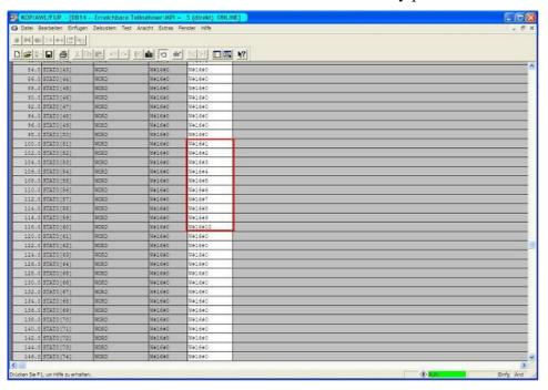
The bytes from DW100 should be the same as the ones you have configured in the DB100 S5 - PLC from DW0.
