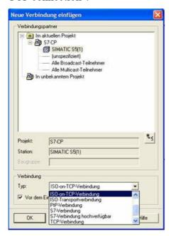
13. Now open the properties of the connection with "OK", where you must now put a "tick" under the "General" in "active connection".
