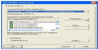
18. If you want to use ProTool/Pro RunTime you can set the "PG/PC Interface" by selecting the entry "DPSONLINE". Therefore you have to select "Access Point of Application" and configure it as described above. The easiest way is to use the S7-LAN/MPI-LAN/MPI-USB- driver which supports USB and LAN products.
