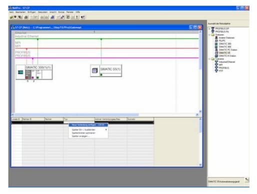
12. Now select here as the connection type the previously configured S5 - PLC and the "ISO-on-TCP connection".
