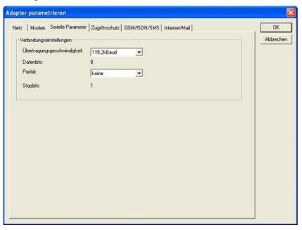
In this dialog the transfer-rate between modem and TS-Adapter is selected.
