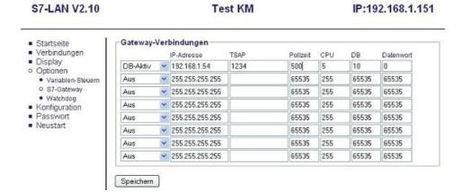
The final step is to configure the gateway. Here you have to set "Connection Type" to "DB - active" and at (the partner device" passive) "Station Number" you must enter the number of your PLC. Now you should decide which is the configuration data block in your PLC and from which data word. The IP - address of your S5 - LAN type in "IP - address partner" field. In "TSAP" you store now have the same name as in the S5 - LAN Manager your S5 - LAN are assigned.
