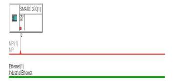
7. Now add a S7-PLC as replacement for S7-LAN/MPI-LAN which will be used for the CP mode later.
