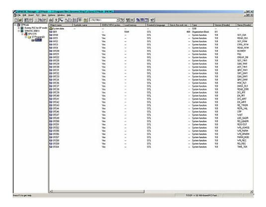
As soon as the blocks are shown, right beside the device explorer, the CP communication with the PLC over the S7-LAN module is established.
