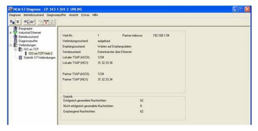
4. For added control, you can now take the DB10 in your S7 - SPS (with CP) and take the DB14 in your S7 - SPS (with S7 - LAN gateway), and check if the values of the 20 bytes you have configure in the each other PLC in DB10 and DB14 from DW0, match with those from DW100. If that is the case, the communication between S7 and S7-CP-LAN was completed successfully.
