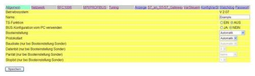
Under "Network" you have to adjust the "DHCP - client" to "OFF" and set the IP - address of the module.
