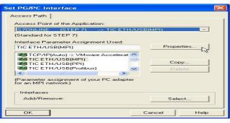
9. Is the device-type is not identical with your used device, search for your device with "Search Device". Select the device in the result windows and click on the button "Apply".
