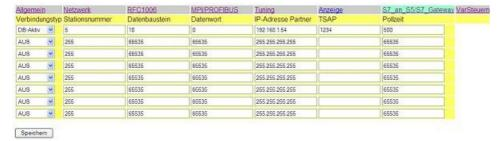
Finally, you still have to enter the number of your CPU that is stored in your PLC about "RFC1006" in "destination - CPU", and the "Bus" should be "Config".
