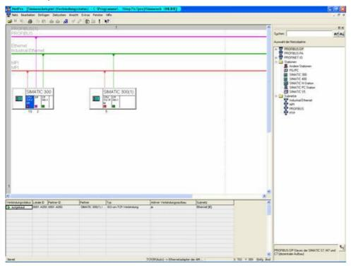
3. Now open as previously mentioned the "diagnostic window" via the object properties of the "CP". There you start the "Cyclic Refresh" and under your observe "ISO-on-TCP connection," the statistics where the sent and received messages are counted. So you can check if your connection is available and also runs.
