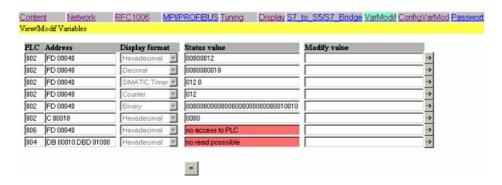
If a password for VarModif defined, you encounter a password check at access to this Dialog, if the password is wrong or not inserted the modification of operand-values is not permitted.
