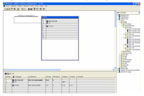
5. Now open the object properties with a right click on your projected CP. Under "General" you can now connect under interfaces these to the Ethernet network and assign an IP to him.
