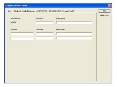
The Access over a telephone-line on the PLC could be configured in this dialog.
