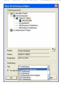
12. With OK now opens the properties of the compound where you have to put a tick under "General" at "active connection".
