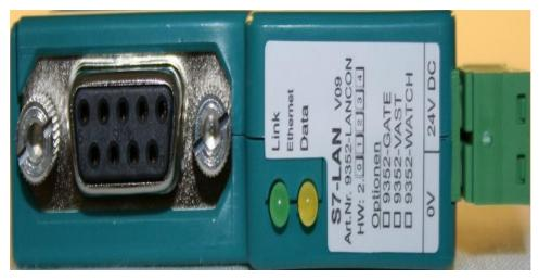
The lateral LEDs behave exactly like the LEDs on the Ethernet socket.
