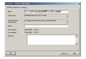
9. Type in the edit box "Name" the new name of the PLC (e.g. "S7-LAN-module/MPI-LAN-cable for CP mode"). Confirm the new name with a click on "OK".
