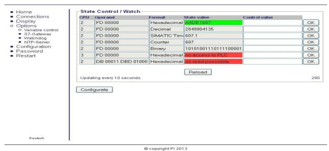
Controlling variables can always be opened with a configured password, and the configured status values can be read out. Do you want at a configured password transferred the control values in the PLC you are asked for the password. At incorrect or missing input the controlling of the variables is not allowed.
