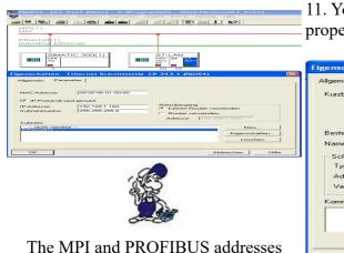
The MPI and PROFIBUS addresses must be 1 less than the address on the back wall of the CP. In this image the MPI and Profibus address is 10 therefore the address on the back panel of the CP is 11
