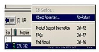
27. In the dialog "Properties – CPU 312 - (R0/S2)" press the "Properties..." button. In the new dialog you can assign the MPI address to the CPU and choose the subnet the CPU should use.
