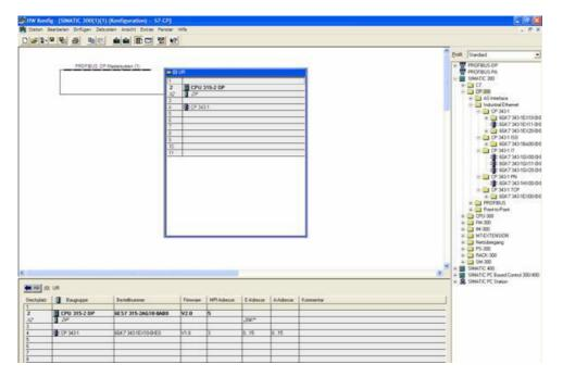
5. Now open the object properties by right-clicking on your configured CP. Under "General", you can now connect these to the Ethernet network under interfaces and assign an IP to him.
