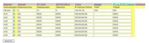
Lastly, you must now enter the number of your CPU that is stored in your PLC under "RFC1006" in "destination - CPU" and the "Bus" should be "Config".
