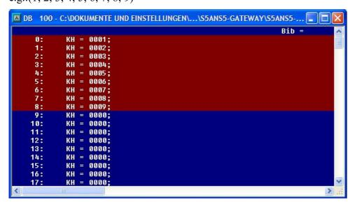
2. Open the DB14 in your S7 - PLC and enter any desired values in the first 20 bytes. e.g.: (1; 2; 3; 4; 5; 6; 7; 8; 9; 10)
