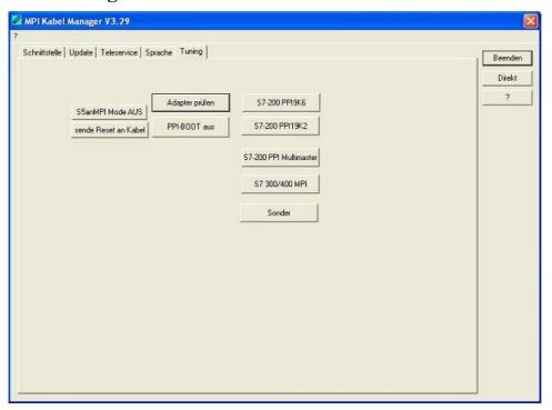
This tab is only used in some special cases. If you press the button "Check Adapter" the cable is connected und after that the following dialog is displayed:
