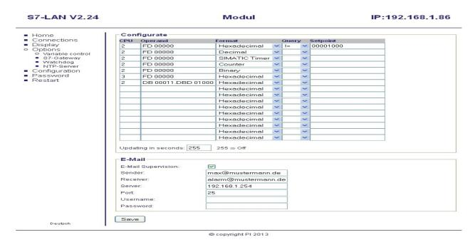
When set to "update in seconds" can the reading in the status values effected cyclically.
