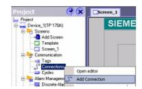
5. A new configuration window "Connections" opens in the right part of the main window. This offers you different setting options.
