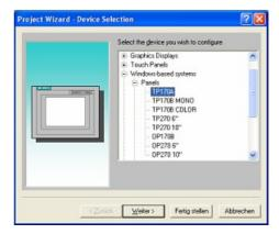
4. "Next" leads you to a new dialog. Type in the specfic fields the name of the PLC device and choose the used PLC in the driver selection (e.g. "SIMATIC S5 – AS511 V6.0")
