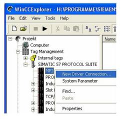
6. For a proper working communication with the PLC there must be defined how the software has to communicate with the PLC
