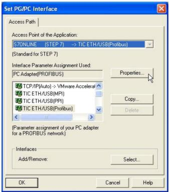
18. If you want to use ProTool/Pro RunTime you can set the "PG/PC Interface" by selecting the entry "DPSONLINE". Therefore you have to select "Access Point of Application" and configure it as described above. The easiest way is to use the S7-LAN/MPI-LAN/MPI-USB- driver which supports USB and LAN products.
