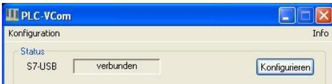
5. After a successful connection, in the main window of the PLC VCOMs appears the cable type with which the computer connects and the connection status is "connected".
