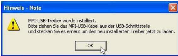
7. After the driver has been installed, please disconnect your MPI-USB Cable and then connect it again.
