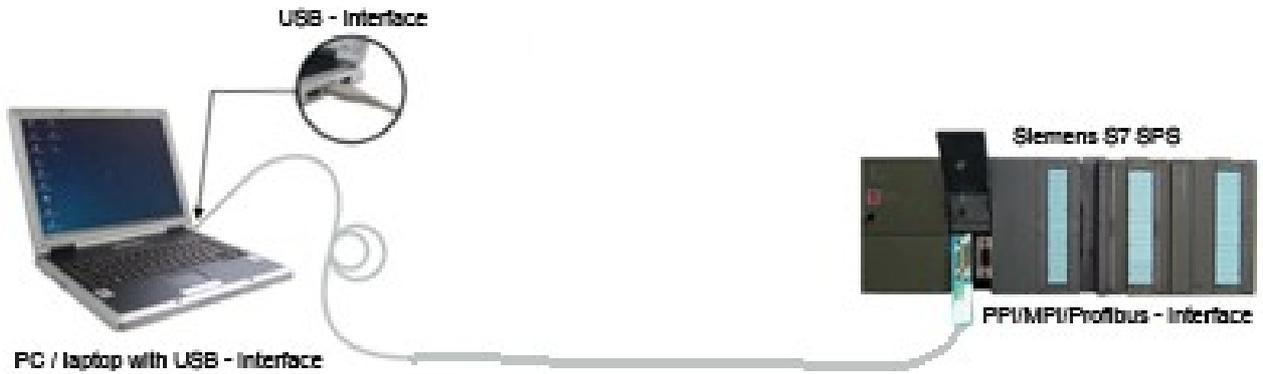
S7-USB connected with PC over USB-Hub.
