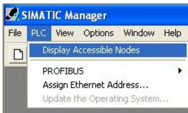
1. Klick in the drop - down menu "target system" on "Display Accessible Nodes".
