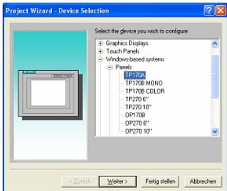
4. „Next“ leads you to a new dialog. Type in the specific fields the name of the PLC device and choose the used PLC in the driver selection (e.g. „SIMATIC S5 – AS511 V6.0“)
