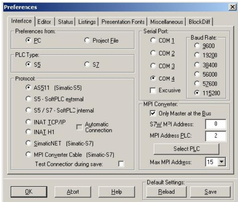
4. Choose the first registry card „Interface“ (standard) and set up the configuration data as described below:
