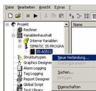
6. For a proper working communication with the PLC there must be defined how the software has to communicate with the PLC
