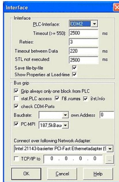
4. Set in the section "Bus grip" the tick "Grip allways only one block from PLC", "FB-names", "Bst. Info" and "check "COM-Ports"
