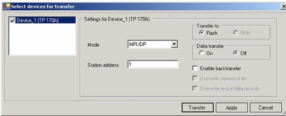
9. Press the button „Transfer“ to start communication with the terminal. Your project is about to be transferred.
