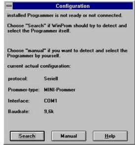
By pressing the operation button "search" the program tries to search and adjust the programmer automatically. First the programmers PG Prommer I, PG Prommer II, Multiprommer, FlashPrommer and Flash-Prommer II are searched on the serial interfaces. After that the MINI Prommer and then the Muliprommer are searched on the first parallel interface. If your programming device shoudn't be recognized, this is due to an inuse USB-Seriell Konverter. Therefor use the manual input!
