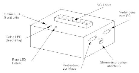
Connect the Mini-Prommer to your PC with the supplied serial connection cable. Connect the 24V power supply with the Mini-Prommer. This now power up automatically and the green LED starts to flash cyclically.
