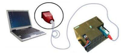
In the first step you should put your LAN device on the PPI/MPI/Profibus interface of your PLC. If a bus cable is already connected to the interface of your PLC you can simply connect your device on top of the cable if a diagnostic jack is available. You can also put your device directly on a slave module (e. g. a panel) if you don't want to work on a bus with a controller.
