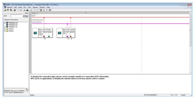
Now you have to add a new "SIMATIC 300" station to your project. This can be selected from the catalog on the left side. Finally you should give the station a suitable name for a better identification.
