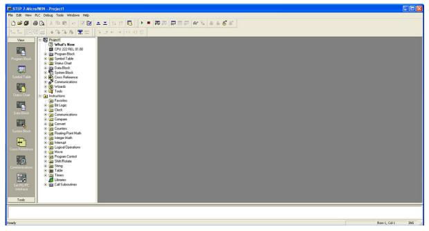
If the interface is configured you will have to set up the communication to the controller. Therefore you have to click on "Communications". This item can also be found within the block "View" on the navigation bar on the left side of the program. After you have clicked on the item you should get the following dialog:
