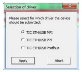
When you have selected a S5-LAN module, the module can be set up for the usage together with the PLC-VCOM. After you have clicked on the button "setup communication", the program will check if the PLC-VCOM is installed on your PC and not to old. After that the TIC will start the PLC-VCOM (if not already started) and then lets the PLC-VCOM connect to the specified device. Next the TIC waits for the response and finally shows you a message with the current state:
