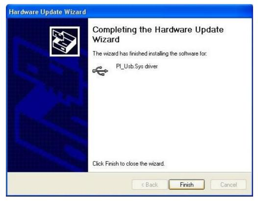
If you want to make sure that the installation of the driver was successful, you can now open the Device Manager and search for the entry "PI\_Usb.Sys driver" within the group "Universal Serial Bus controllers".
