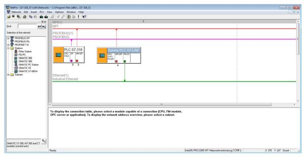
In one of the last steps you should save and compile the configuration again. If an error while compiling occur you should check all done settings again. Otherwise the configuration can be downloaded to the real existing controller. The transmission of the configuration to the Dummy PLC isn't possible and also don't needed.
