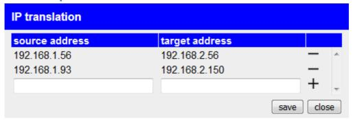
If the IP switch option is available and activated in your device, you have the option to set the IP address conversions for the peripheral interface devices in the "IP Conversion" dialog. The source address is the original IP address of the devicethe peripheral interface. The target address describes the address into which this IP address should then be converted.
