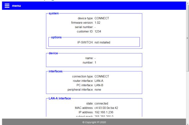
The "Status" page shows various status information about the device as well as the device's settings and network interfaces. This information may be helpful if you, for example, For example, you want to check whether the device has established an LTE or WLAN connection and how good the signal level is. If you have problems with the device, this information may also be helpful for support.
