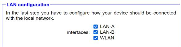
In the final commissioning step, you determine which interfaces should be connected to a common network as a bridge and represent the local network (LAN). Depending on your needs, you can choose one or more interfaces here.
