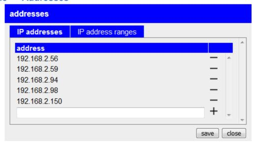
The "Addresses" dialog allows you to configure the addresses or even entire address ranges for the peripheral devices. The address configuration is divided into several tabs, with only the "IP addresses" and "IP address ranges" tabs currently available. The respective list can be opened by clicking on the tab.
