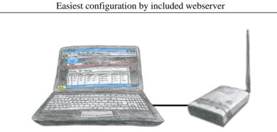
To configure ALF you dont need additional driver or special cables, you connect your PC via LAN or WLAN with ALF and over the integrated webserver you can configure the needed function.
