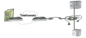
You have to reach urgend your PLC via remote maintenance and have no TS-adaptor in your company? No problem, configure with the MPI-Kabelmanager your S7-interface-cable MPI-II-Kabel the mode "TS" for "remote maintenance", connect this cable with the TS-Adapter (article number 9350-TS) with a standard modem and send it all to your client. Now you will be able to start the connection with your TS-sofware and solve the problem. And this all without buying a original TS-adapter.
