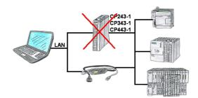
Do you have a S7-PLC-device without CP243-1, CP343-1 or CP443-1 and would like to connect via LAN? Then plug the S7-LAN on the PLC-device and your access via RFC1006 is ready for use.
