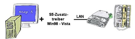
You still have a PC with Win98 and a MS-DOS-based Step5-package and would like to go Online on your S5-PLC via LAN? No problem, the provided virtual Com-Port PLCVCom emulates a COM-port on your PC with which you go Online. Even your MS-DOS-based Step5-software on this WIN98-PC can use this virtual Com-Port. With a patchtool for the Siemens Step5-software, which is provided as well, nothing else stands in your way to communicate via LAN.
