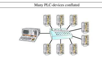
You have many PLC and you want to programm them central on one place? No problem, you have to connect them all to the KOR/MUX-Tele-Switch an with the PD-bus-selection of your Step5-software you go ONLINE. Of course the KOR/MUX-Tele-Switch is cascadable, so you can connect up to 30 PLCs to the devices.
