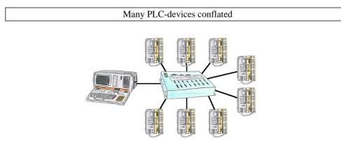
You have many PLC and you want to programm them central on one place? No problem, you have to connect them all to the KOR/MUX-Tele-Switch an with the PD-bus-selection of your Step5-software you go ONLINE. Of course the KOR/MUX-Tele-Switch is cascadable, so you can connect up to 30 PLCs to the devices.
