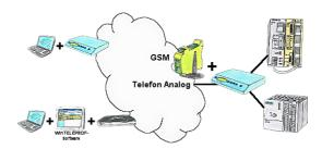
Access to the connected PLC takes place by coupling via Analogue-, ISDN- (only with AB-adapter) and GSM-(only with external GSM-modem)-line.
