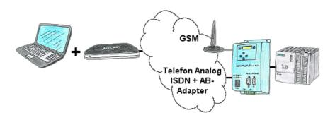
The access to the connected PLC with the Siemens TS-software or PG-2000 including TS-option results of coupling via Analogue-, ISDN- (only with AB-adapter) as well as GSM-line.
