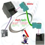
Direct data-exchange between S7-PLCs with S7-LAN.
