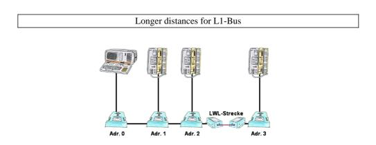
You need for your L1-Bus higher distance like the possible 1200m? You have strong distrubance on your L1-Bus? You need a serial line for higher distances and this galvanic decoupled? No problem, all this points are solved through the LWL-adapter. They are available for artificial and optical fibre, for L1-Bus and RS232.
