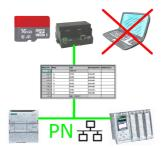
S7-PLC triggered DB-backup/-restore without additional PC via PN-port on SD card
