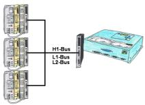
You have an existing L1-, L2- or H1-bus on the customer side and have to program parallel the PLCs? No problem, just connect the communication processor (CP) with a monkey swing to the PLC, the Tele-Network-device with the TELE-CP-cable to a free CP and select the needed PLC with PG-path selection. Herefore the L1-, L2- or H1-option is needed.
