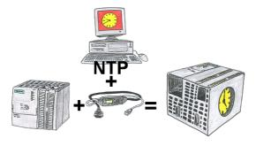
You need in your PLC a actual time? No problem, with the NTP-function the MPI-LAN-cable get from a NTP-(Time-)Server the actual time and transfers it direct into the configured PLC or for processing in a DB.
