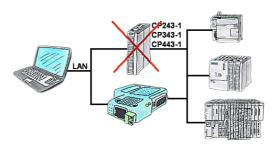
Do you have a S7-PLC-device without CP243-1, CP343-1 or CP443-1 and would like to connect via LAN? Then plug the S7-LAN on the PLC-device and your access via RFC1006 is ready for use.
