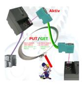
Direct data-exchange between S7-PLCs with S7-LAN.
