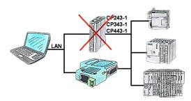
Do you have a S7-PLC-device without CP243-1, CP343-1 or CP443-1 and would like to connect via LAN? Then plug the S7-LAN on the PLC-device and your access via RFC1006 is ready for use.
