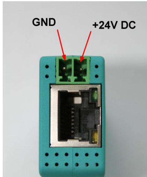
**Before using the external power supply, check the correct pinning of the Phoenix plug! The module itself is protected against wrong pinning the phoenix plug, but we can not guarantee for protection for the possible connected assemblies.**
