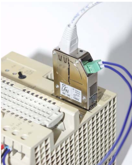
S5-LAN connected to SIMATIC S5 plc 95U
