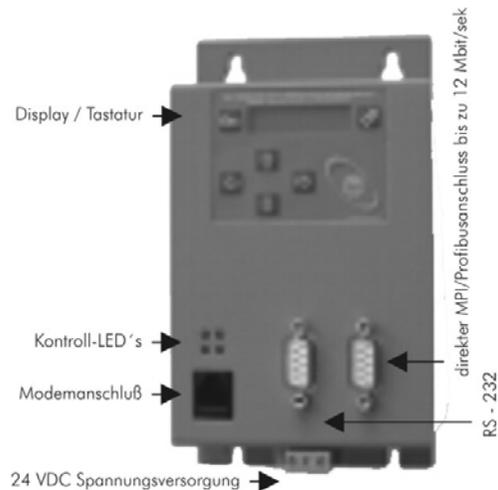
In the version "ohne Profibus" there are baudrates until to 12MBaud (MPI and programming over profibus), but not DP V0 / V1 / V2
